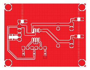
Figure 4: AAT4626 Evaluation Board Component Side Layout.
