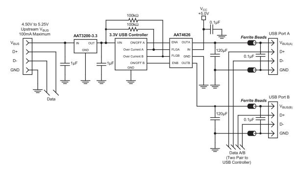
Figure 8: Self-Powered Dual Port USB Hub.
