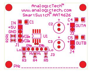
Figure 6: AAT4626 Evaluation Board Top Side Silk Screen Layout /Assembly Drawing.
