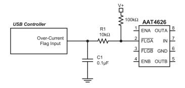
Figure 1: Fault Flag Delay RC Filter.
