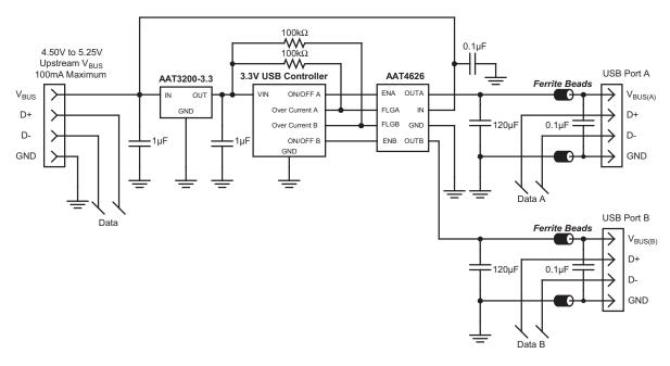
Figure 9: USB Bus Powered Dual Port USB Hub.
