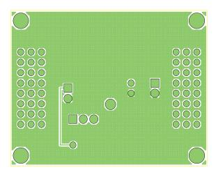
Figure 5: AAT4626 Evaluation Board Solder Side Layout.
