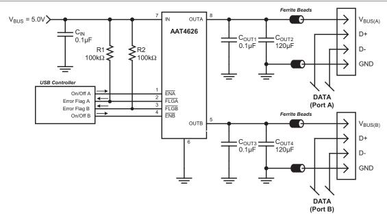
Figure 7: Typical Dual USB Host Port Application.
